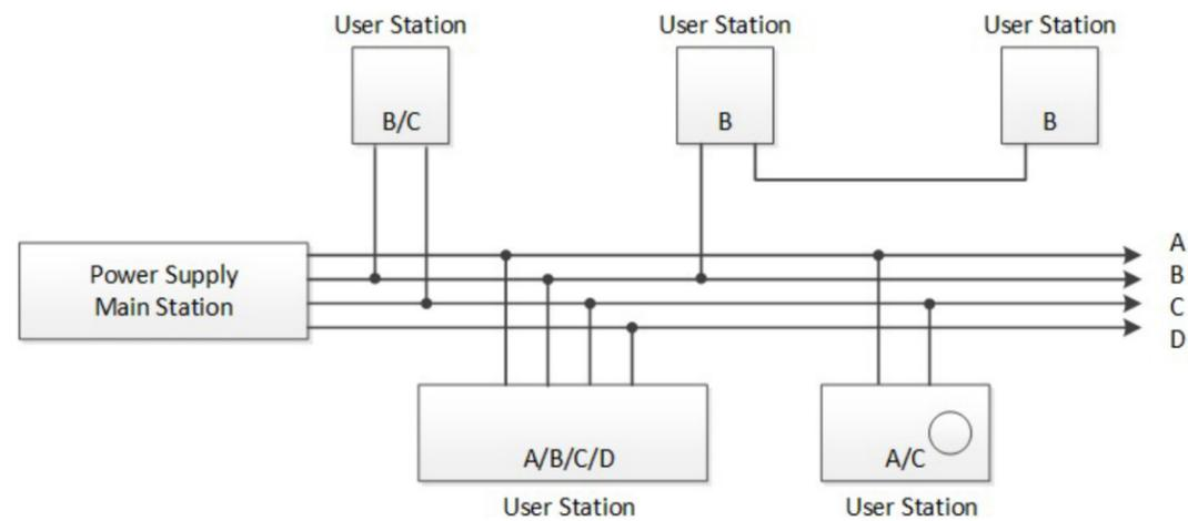
Figure 1: 4 - Channel Clear-Com Concept using Single Twisted Pair Shielded Cable
